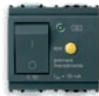
16511.10 C 10, I \Delta n 10 mA p.i. 3000 A - 2 moduli
