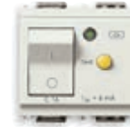
16511.16.6 C 16, I \Delta n 6 mA p.i. 3000 A - 2 moduli
